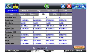
For advanced troubleshooting, Upstream Pre-Equalization Adaptive EQ parameters and In Channel Frequency Response can be viewed by tapping on the desired UCD number.
